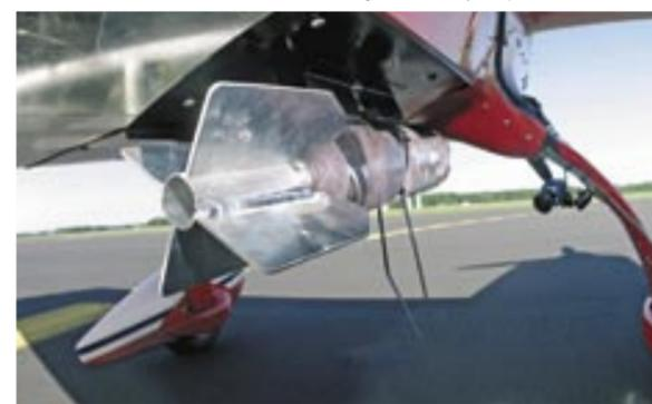
**ABOVE** Most competitors modified their aircraft to drop the bomb from a release mechanism beneath the fuselage.
